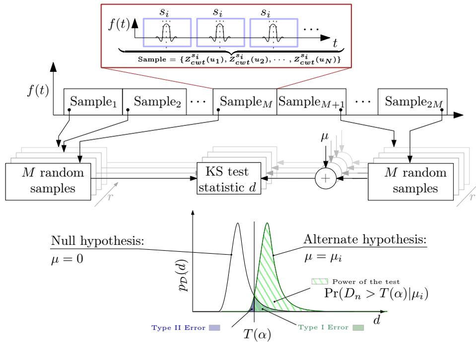
Figure 5: The scheme for empirical evaluation of the power of the KS test. The critical value  $T(\alpha)$  of the test determines the boundaries of the acceptance region  $[0, T(\alpha)]$  of the test where  $\Pr(D_n > T(\alpha) | \mu = 0)$  equals to the significance level  $\alpha$ .
