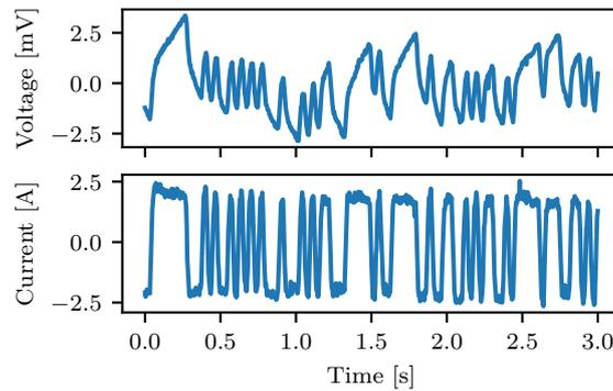
Figure 8: A sample of the current probing signal and the resulting cell voltage signal acquired during an experiment
