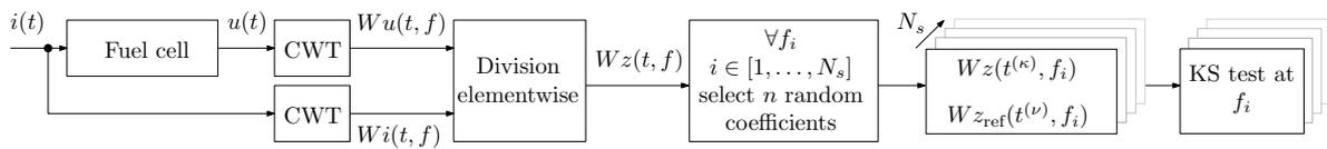
Figure 6: Evaluation scheme for performing the two-sample KS test using CWT coefficients for each frequency (scale)  $f_i$ . Time moments  $t^{(\kappa)}$  and  $t^{(\nu)}$  are sets of  $n$  randomly chosen time instances within the observation window and may generally differ among different frequencies.
