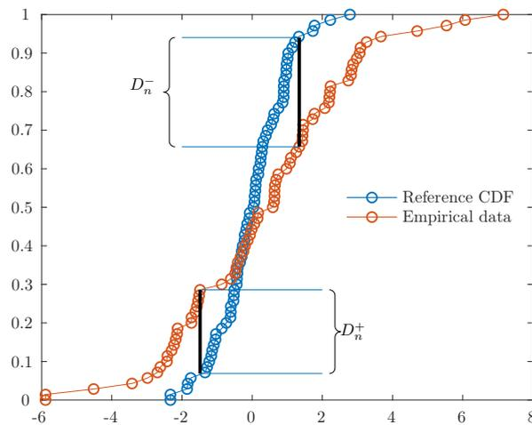
Figure 4: The comparison of two empirical distributions obtained from two samples of different population illustrates the value of the one-sided two-sample KS test statistic  $D_n^+$  or  $D_n^-$ . Each empirical distribution is obtained from  $n = 70$  realisations of two independent, normally distributed random variables with zero mean and unequal  $\sigma$ : the standard deviation in the blue and red colour corresponds to 0.2 and 2, respectively.
