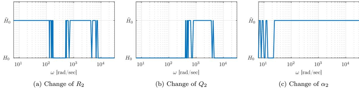
Figure 7: Frequency regions where null hypothesis  $H_0$  can be rejected based on the KS test on the numerical example for system (3)
