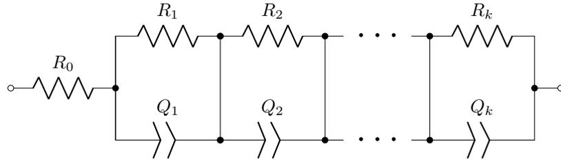
Figure 2: Schematic representation of the ECM (2)
