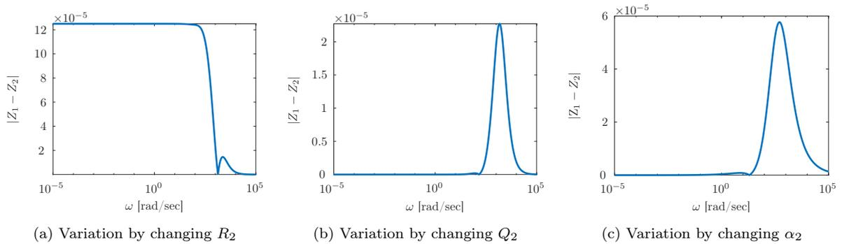
Figure 3: Module of differential impedance  $|\Delta Z| = |Z(\theta + \Delta\theta)| - |Z(\theta)|$  where  $\theta \in (R_2, Q_2, \alpha_2)$
