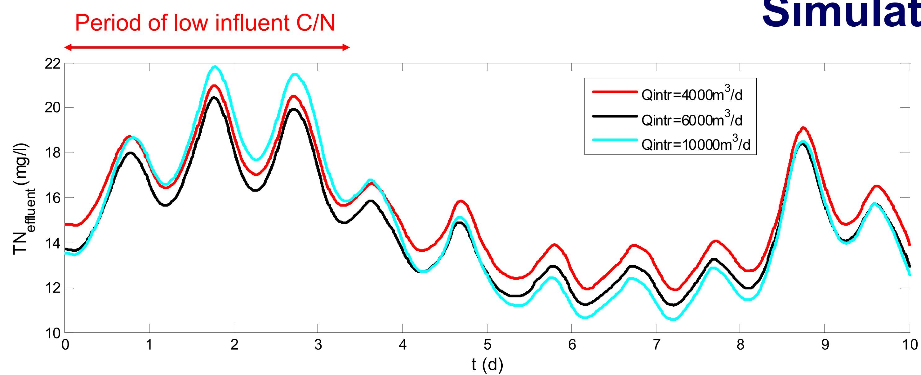
Simulations with different constant nitrate recirculation flows ( $Q_{\text{intr}}$ ) were performed using a pilot plant simulation model and dynamic real plant influent data.
