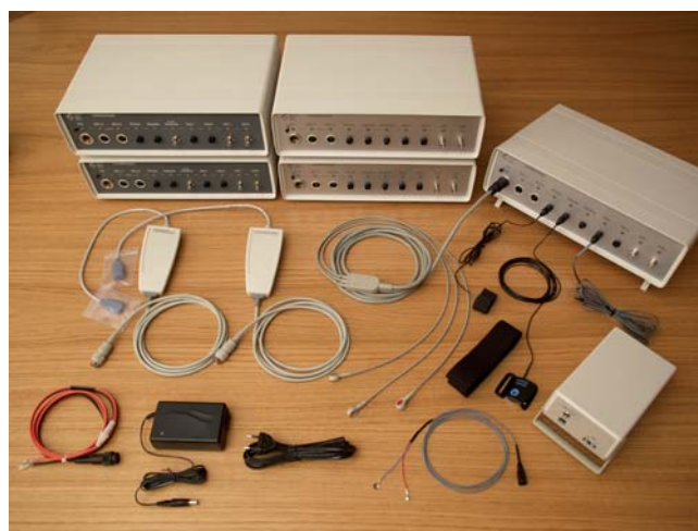
Figure 5: The Cardio&BrainSignals 12-channel measurement system, which enables the measurement of ECG, EEG, respiratory effort, blood pressure, skin conductivity, high-resolution temperature and two auxiliary channels
