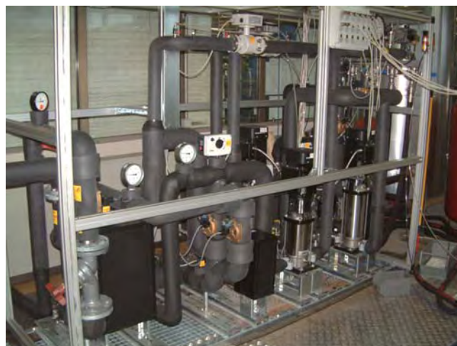
Figure 5. Semi-industrial setup for systematic functional testing of elements needed in the heating and climatisation of buildings. The control system for the setup shown here was developed by the Department of Systems and Control.
