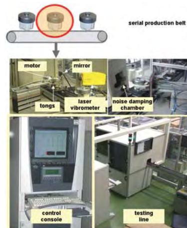
Figure 3: System for automatic final quality control of vacuum cleaner motors in the company Domel, Želeniki, Slovenia.
