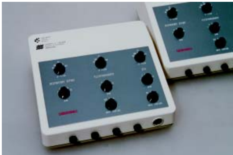
Figure 2: "Cardiosignals" - A signal conditioning system for the acquisition of physiological signals
