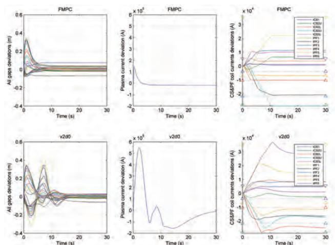
Figure 1: Simulation performance comparison between the MPC plasma current and shape control (top) and the reference CREATE v2d0 scheme (bottom): minor disturbance at  $t = 520$  s. Left: plasma edge geometrical descriptors, centre: plasma current, right: poloidal field coil currents (dotted lines: constraints, with triangles marking their directions)
