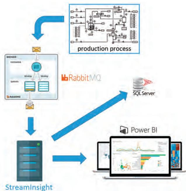
Figure 2: The architecture of the environment for complex data processing
