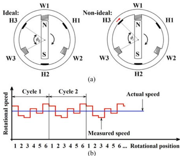
Fig. 1. (a) Schematic of the BLDC motor: stator windings are denoted by W1, W2, and W3, rotor is N-S, Hall sensors H1, H2, and H3 are positioned ideally and nonideally, respectively. (b) Actual rotational speed (ideal) and measured rotational speed (nonideal).
