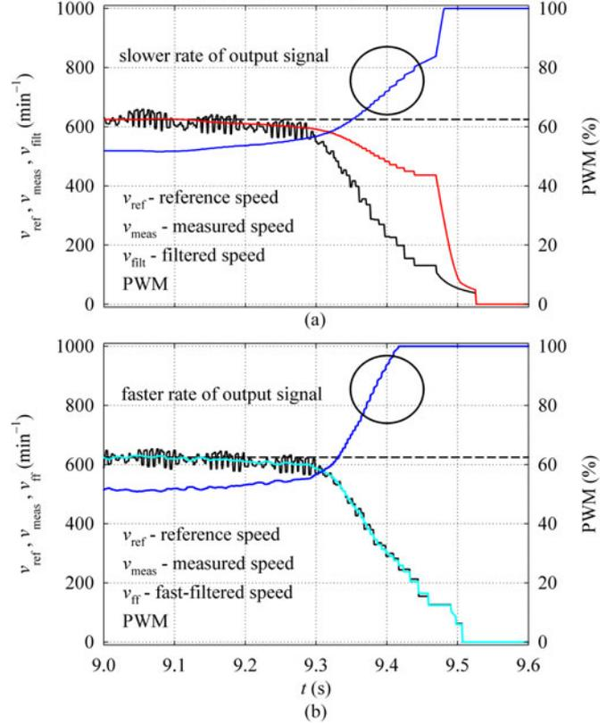
Fig. 12. Reference ( $v_{\text{ref}}$ ), measured ( $v_{\text{meas}}$ ), filtered ( $v_{\text{filt}}$ ), and fast-filtered ( $v_{\text{ff}}$ ) rotational speed of the BLDC motor as a function of time  $t$  when reaching the end position. (a) Filtered speed and (b) fast-filtered speed is used as PID controller's input. The output signal of PID controller is PWM ratio.
