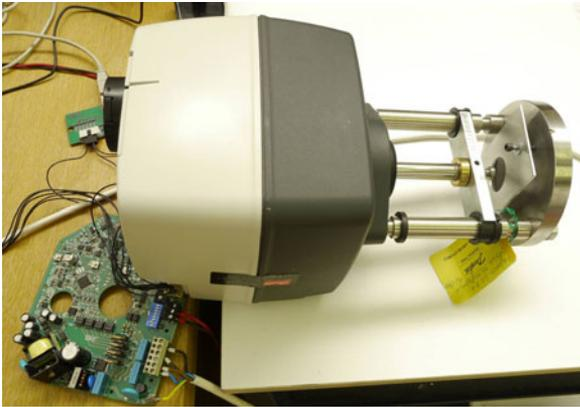
Fig. 6. Valve actuator with prototype electronics.
