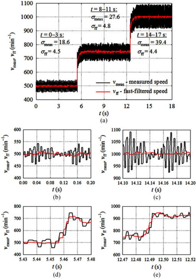
Fig. 9. (a) Measured ( $v_{meas}$ ) and fast-filtered ( $v_{ff}$ ) speed as a function of time ( $t$ ) when the  $v_{ref}$  is abruptly increased by increments of  $250 \text{ min}^{-1}$  from  $500 \text{ min}^{-1}$  to  $1000 \text{ min}^{-1}$  with corresponding standard deviations ( $\sigma_{meas}$  and  $\sigma_{ff}$ , respectively) in the steady-state conditions. (b) and (c) Detailed view of  $v_{meas}$  and  $v_{ff}$  under steady-state operation and (d), (e) during transients.
