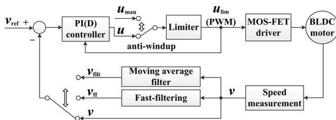
Fig. 7. Schematic of the rotational speed control loop.
