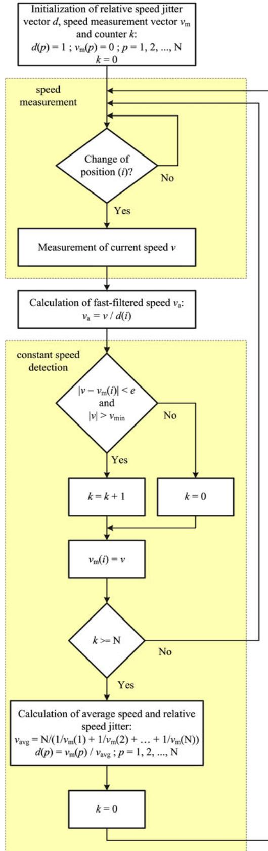
Fig. 4. Schematic diagram of the proposed fast-filtering algorithm.
