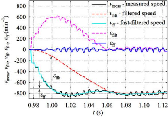
Fig. 11. Measured ( $v_{\text{meas}}$ ), filtered ( $v_{\text{filt}}$ ), and fast-filtered ( $v_{\text{ff}}$ ) rotational speed of the BLDC motor, after running to backward rotational direction, as a function of time  $t$ . The difference between  $v_{\text{filt}}$  and  $v_{\text{meas}}$  and the difference between  $v_{\text{ff}}$  and  $v_{\text{meas}}$  is denoted with  $\varepsilon_{\text{filt}}$  and  $\varepsilon_{\text{ff}}$ , respectively.
