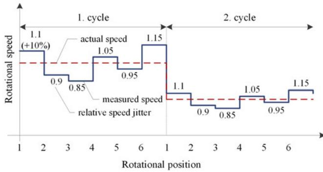
Fig. 3. Actual and the measured speed with relative speed jitter at different rotational positions.
