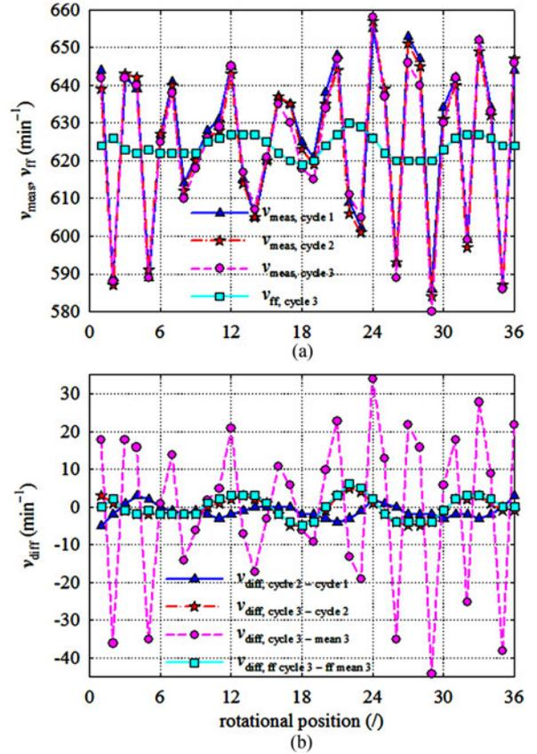
Fig. 10. (a) Measured ( $v_{meas}$ ) and fast-filtered ( $v_{ff}$ ) speed. (b) Their mutual differences ( $v_{diff}$ ) as a function of rotational position within three consecutive rotational cycles.
