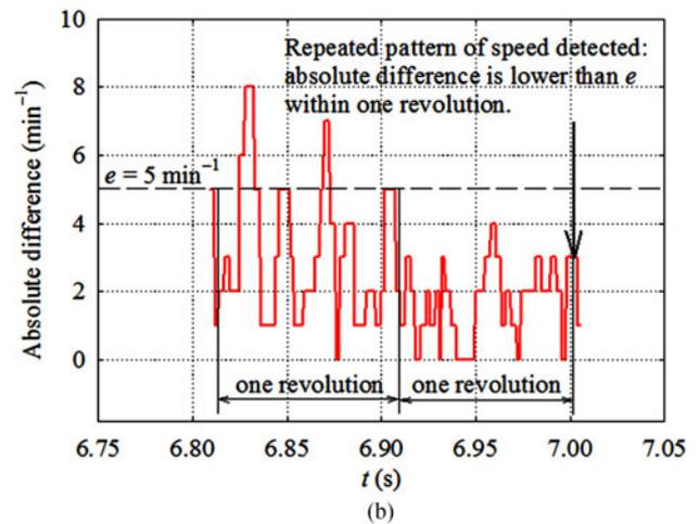
Fig. 8. (a) Reference ( $v_{\text{ref}}$ ), measured ( $v_{\text{meas}}$ ), and fast-filtered ( $v_{\text{ff}}$ ) rotational speed of the BLDC motor after the microcontroller's reset. (b) Absolute difference of measured speed samples between two consecutive full revolutions of BLDC rotor, as a function of time  $t$ .
