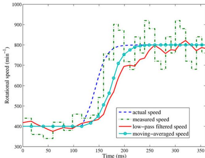
Fig. 2. Actual, measured, low-pass filtered, and moving-averaged speed in revolutions per minute ( $\text{min}^{-1}$ ).
