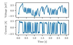
Figure 8: A sample of the current probing signal and the resulting cell voltage signal acquired during an experiment
