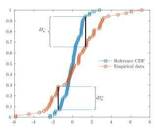
Figure 4: The comparison of two empirical distributions obtained from two samples of different population illustrates the value of the one-sided two-sample KS test statistic  $D_n^+$  or  $D_n^-$ . Each empirical distribution is obtained from n = 70 realisations of two independent, normally distributed random variables with zero mean and unequal  $\sigma$ : the standard deviation in the blue and red colour corresponds to 0.2 and 2, respectively.
