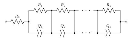
Figure 2: Schematic representation of the ECM (2)
