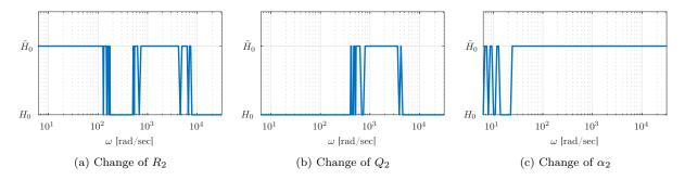
Figure 7: Frequency regions where null hypothesis  $H_0$  can be rejected based on the KS test on the numerical example for system (3)
