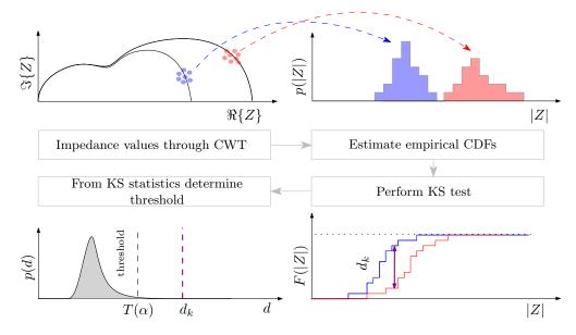
Figure 1: Schematic representation of the proposed approach
