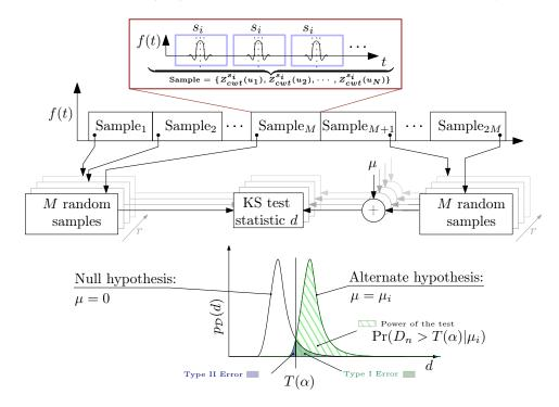
Figure 5: The scheme for empirical evaluation of the power of the KS test. The critical value  $T(\alpha)$  of the test determines the boundaries of the acceptance region  $[0, T(\alpha)]$  of the test where  $\Pr(D_n > T(\alpha)|\mu = 0)$  equals to the significance level  $\alpha$ .
