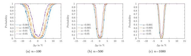
Figure 9: Empirical power of the test for three different sample sizes n and four different significance levels  $\alpha$
