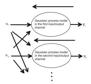
Fig. 1. Principial scheme of modelling multipleinput multiple-output scheme with flow of data used for modelling is indicated
