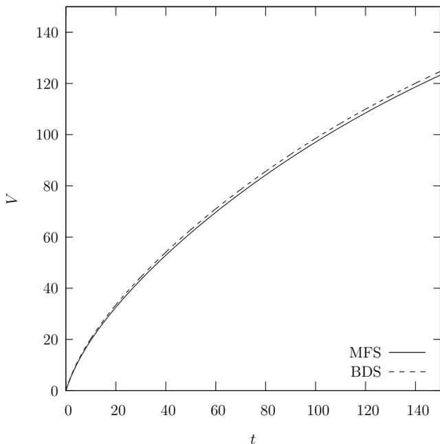
Figure 15: Case 3: Volume as a function of time, comparison between MFS and BDS. The parameters are  $X = 100, Y = 97, R = 1, H = 4, \Delta h = 2, t = 150, N = 181, \Delta x = 2, s = 5, r_0 = \Delta x/4, \Delta t = 0.1$ .
