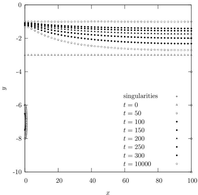
Figure 12: Case 3: The shape of  $\Omega$  at different  $t$  calculated using MFS.  $\Omega$  is delimited by boundary points, the singularities are outside  $\Omega$  and fall outside the graph except in the conduit along the left edge (the circular conduit is not circular in the figure due to different  $x$  and  $y$  scaling). The parameters are  $X = 100, Y = 97, R = 1, H = 4, \Delta h = 2, N = 181, \Delta x = 2, s = 5, \Delta t = 0.1$ .
