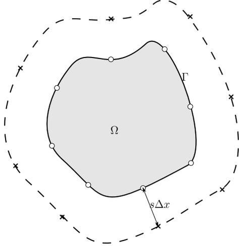
Figure 2: Concept of MFS. Small white circles are collocation nodes with specified boundary condition, crosses are the fundamental solution singularities, and the dashed line is artificial boundary  $s\Delta x$  away from geometrical boundary.
