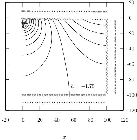
Figure 10: Case 3: Potential  $h$  at  $t = 150$ , calculated using MFS. The other parameters are  $X = 100, Y = 97, R = 1, H = 4, \Delta h = 2, N = 181, \Delta x = 2, s = 5, \Delta t = 0.1$ . The lines represent constant  $h$  and are spaced 0.05 apart. The boundary points are denoted by circles and the crosses mark the poles of the fundamental solutions.
