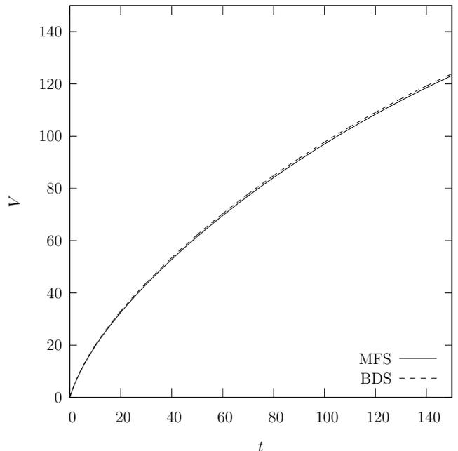
Figure 16: Case 3: Volume as a function of time, comparison between MFS and BDS. The density of the boundary points is larger than in Fig. 15, the parameters are  $X = 100, Y = 97, R = 1, H = 4, \Delta h = 2, t = 150, N = 329, \Delta x = 1, s = 5, r_0 = \Delta x/4, \Delta t = 0.1$ .
