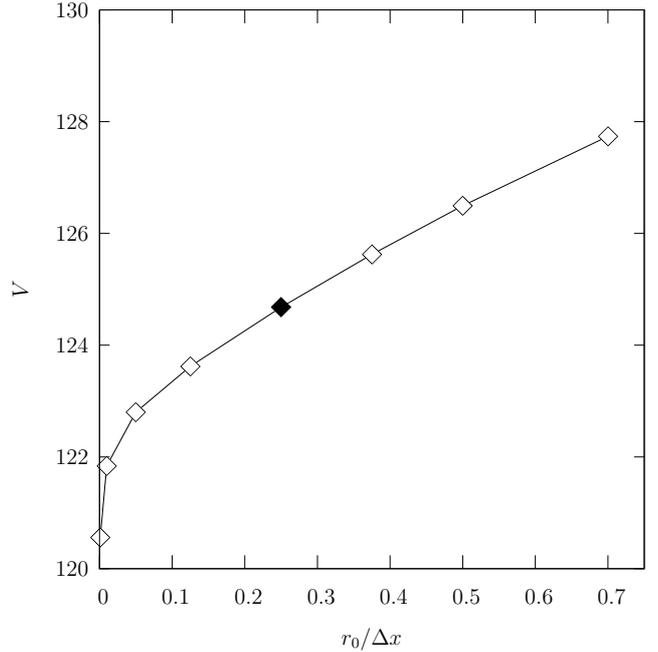
Figure 18: Case 3: Influence of the source radius  $r_0$  on the BDS method. The other parameters are  $X = 100, Y = 97, R = 1, H = 4, \Delta h = 2, t = 150, N = 181, \Delta x = 2, \Delta t = 0.1$ . When  $r_0$  changes for a factor of 700, the change in the result is a few percent. The full diamond corresponds to the standard example.
