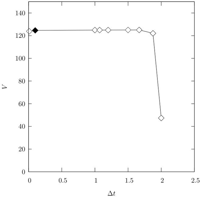
Figure 17: Case 3: Influence of the timestep on the BDS method. The other parameters are  $X = 100, Y = 97, R = 1, H = 4, \Delta h = 2, t = 150, N = 181, \Delta x = 2, r_0 = \Delta x/4$ . It can be seen that the results are fairly consistent up to  $\Delta t = 1.875$  while at  $\Delta t = 2$  the result is obviously incorrect. The full diamond corresponds to the standard example.
