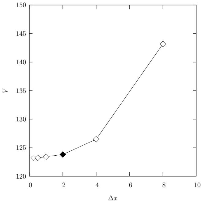
Figure 19: Case 3: Influence of the boundary point spacing  $\Delta x$  on the BDS method. The other parameters are  $X = 100, Y = 97, R = 1, H = 4, \Delta h = 2, t = 150, r_0 = \Delta x/4, \Delta t = 0.1$ . The number of boundary points varies from  $N = 41$  for  $\Delta x = 8$  to  $N = 1202$  for  $\Delta x = 0.25$ . The result is changing slowly as a function of  $\Delta x$  and is steady for  $\Delta x \rightarrow 0$ . The full diamond corresponds to  $\Delta x$  of the standard example.
