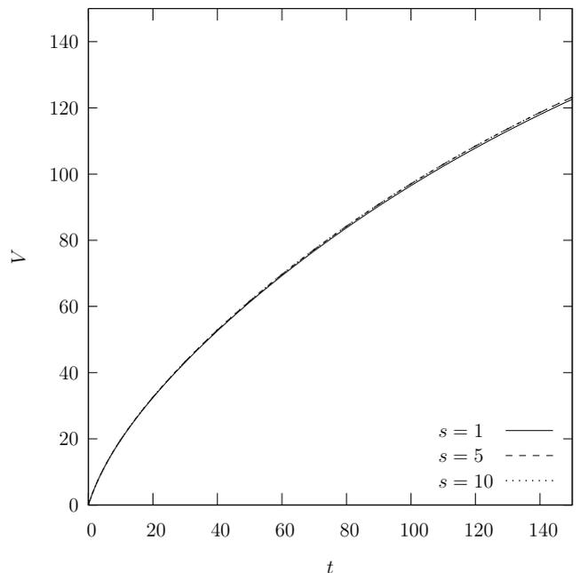
Figure 14: Case 3: Volume as a function of time, calculated for different  $s$  in MFS. The other parameters are  $X = 100, Y = 97, R = 1, H = 4, \Delta h = 2, t = 150, N = 181, \Delta x = 2, \Delta t = 0.1$  as in the standard example.
