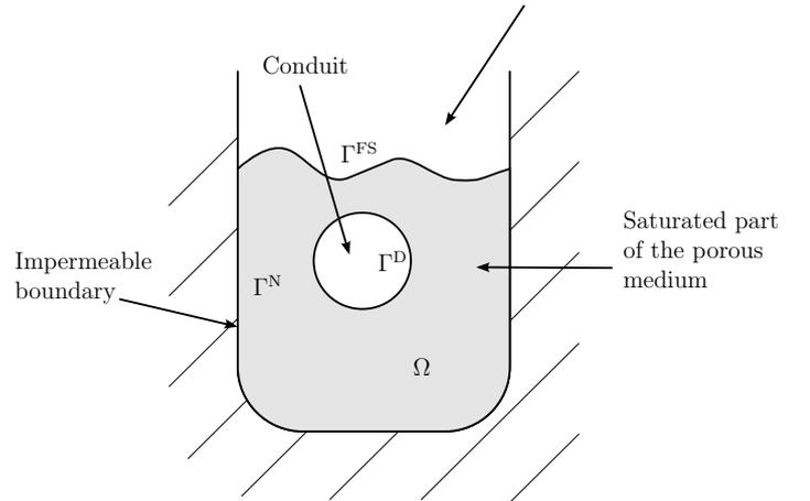
Figure 1: Schematics of the problem domain and the boundary conditions.
