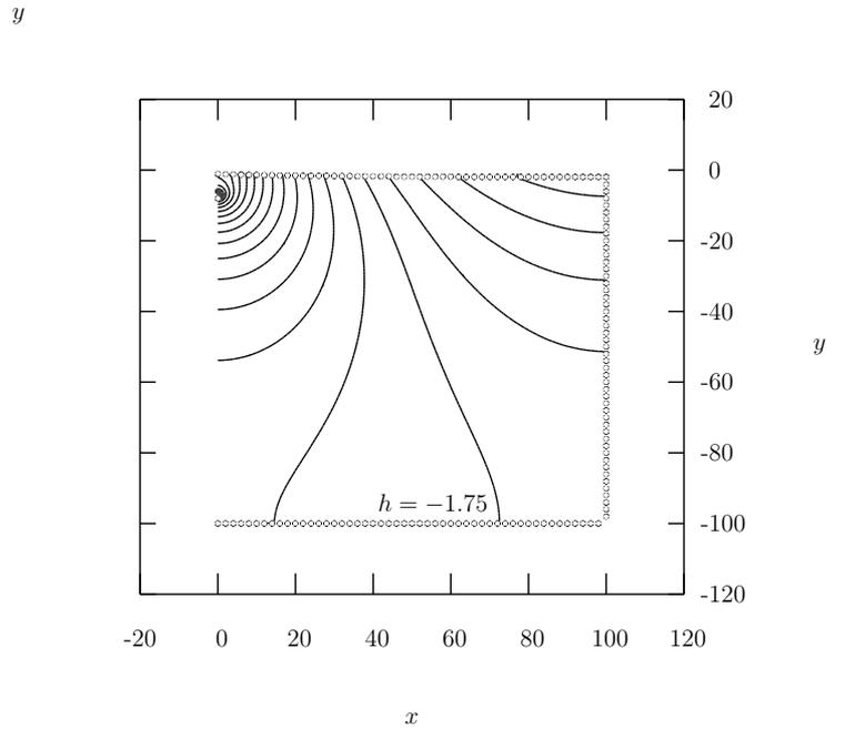
Figure 11: Case 3: Potential  $h$  at  $t = 150$ , calculated using BDS. The other parameters are  $X = 100, Y = 97, R = 1, H = 4, \Delta h = 2, N = 181, \Delta x = 2, \Delta t = 0.1, r_0 = \Delta x/4$ . The lines represent constant  $h$  and are spaced 0.05 apart. The boundary points are denoted by circles.
