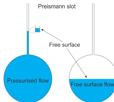
**Figure 4.** The use of a Preissmann slot enables use of the same set of equations for conduits with free-surface flow and conduits with pressurized flow.
