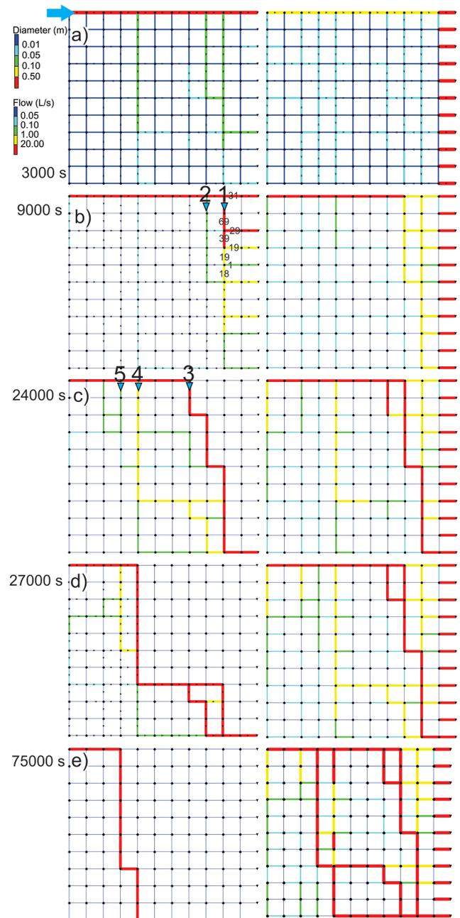
**Figure 18.** High-dip network with random initial distribution of conduit diameters. Flow enters at the top-left edge of the network as pointed by a blue arrow. Values on (b) show flow rates along the selected individual conduits.
