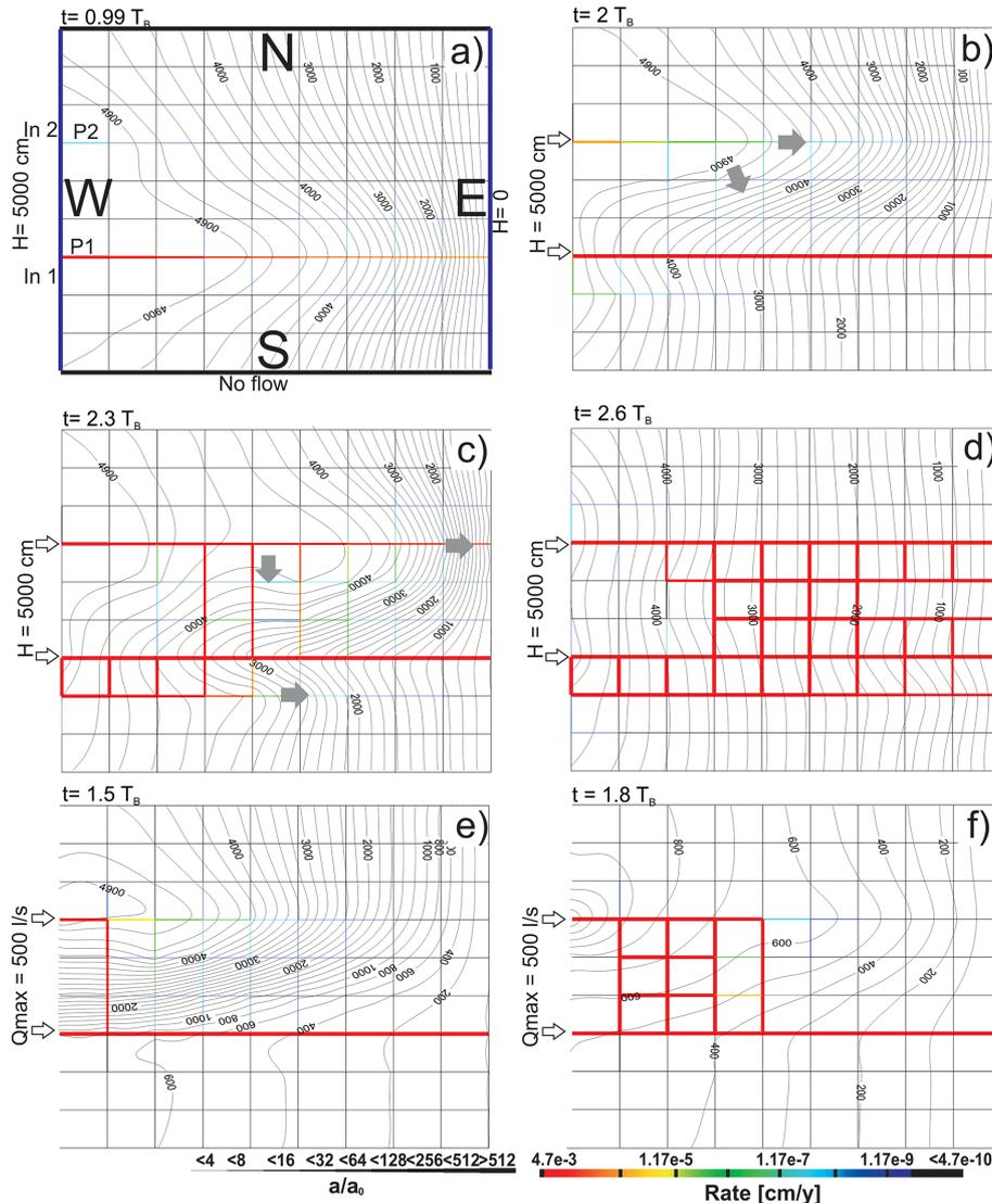
**Figure 1.** Evolution of 2-D fracture network under pressurized flow. Panels show aperture widths and dissolution rates at different stage of evolution. Size of the domain is  $1\text{ km} \times 1\text{ km}$ , initial aperture width  $a_0 = 0.02\text{ cm}$ , except for the line P1, where  $a_0 = 0.03\text{ cm}$ . Linear and fourth order dissolution kinetics for the limestone is used (see Dreybrodt et al., 2005 for details).
