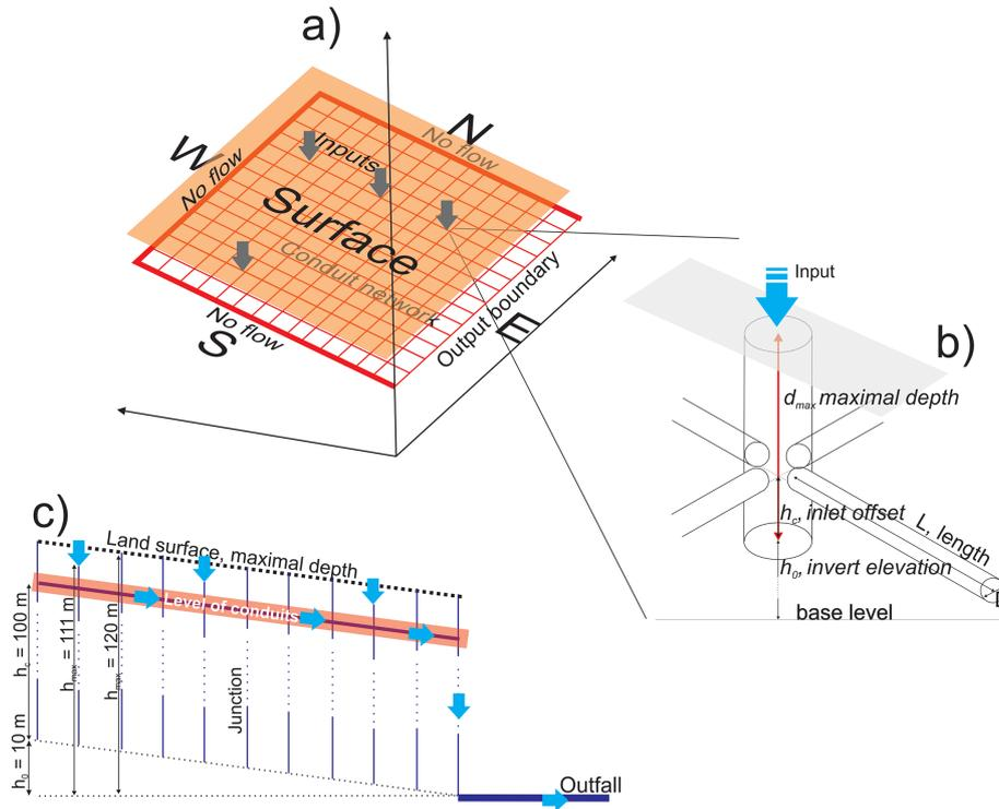
**Figure 6.** The model structure for the low-dip network. (a) A conduit network with discrete water inputs, marked by arrows. Boundaries are denoted geographically. Outputs are along the E boundary. (b) Geometry and parameters of a junction. (c) The side view of the model, also showing a large conduit connecting E junctions to an outfall.
