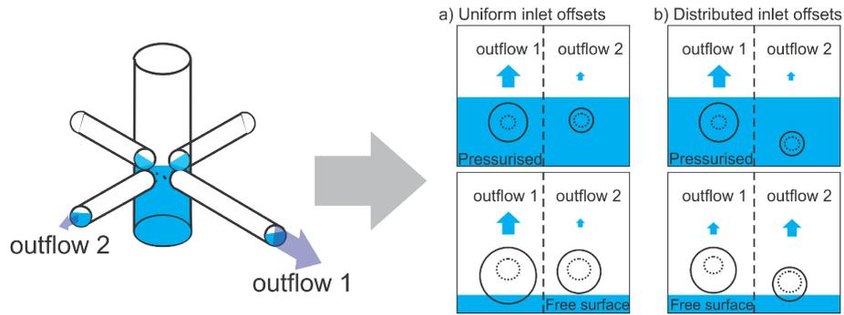
**Figure 9.** Left panel: the geometry of a junction. Right panels (a, b): scheme of two outflows during pressurized flow (top panels) and free-surface flow (bottom panels). (a) Initial inlet offsets for both outflows are equal. (b) Initial inlet offset of outflow 2 is smaller so that the outflow has a lower elevation. Blue arrows indicate the amount of flow drained by each outflow, and the blue shading indicates the water table.
