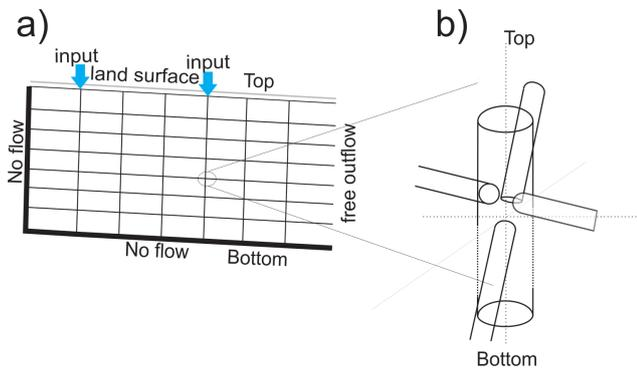
**Figure 7.** The model structure for the high-dip scenario. (a) The slope of the network is 0.99 in from top to bottom and 0.1 from left to right. The right boundary is a seepage face with free outflow. Inputs are on the top. (b) Junction geometry: high-dip (vertical) conduits are positioned below the low-dip (horizontal) conduits.
