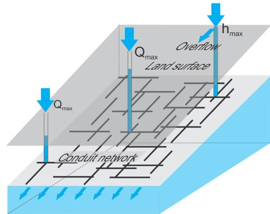
**Figure 3.** Conceptual framework. A conduit network with point recharge at selected locations indicated by arrows. Recharge is limited by the position of the land surface  $h_{\max}$  or by maximal available recharge  $Q_{\max}$ .
