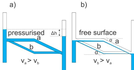
**Figure 14.** Distribution of flow between two pathways depends on the flow resistance when the flow is pressurized. The pathway *a* has with lower flow resistance grows faster. After the transition to free-surface flow, the pathway *b* with higher exit slope from the junction can capture more flow and incise faster.
