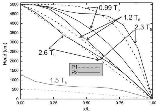
**Figure 2.** Profile of hydraulic head along pathways P1 (dashed lines) and P2 (full lines) from Fig. 1. Profiles are taken at different time steps, given in units of breakthrough time ( $T_B$ ). Gray lines show scenario with constant input at  $1.5 T_B$  (Fig. 1e).
