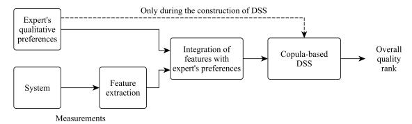
Fig. 1: Structure of the end-quality assessment system
