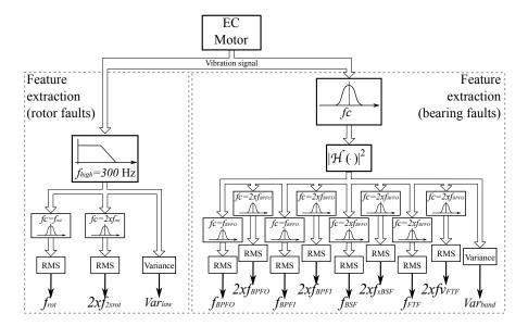
Fig. 3: Structure of the feature extraction module
