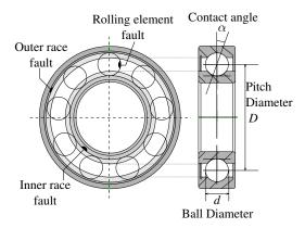
Fig. 2: Bearing dimensions used for the calculation of the bearing's characteristic frequencies
