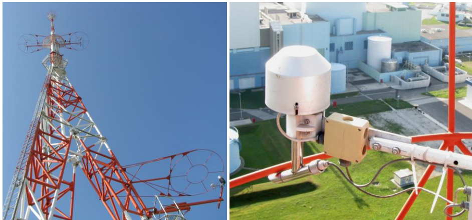
Figure 2. 70-meter-tall tower at measuring site nearby NPP Krško (left: view from ground, right: air temperature sensor mounted at the height of 70 m)
