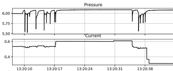
Fig. 5. Pressure and current measurements on EOL testing station – one run.
