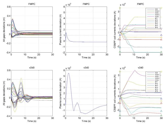
Fig. 3. Simulation performance comparison between the MPC PCSC (top) and the reference CREATE v2d0 scheme (bottom): minor disturbance at t = 520 s. Left:  $\delta \mathbf{g}$ , centre:  $\delta I_p$ , right:  $\delta \mathbf{I}_{PF}$  (dotted lines: constraints, with triangles marking their directions)
