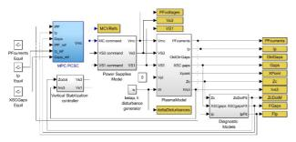
Fig. 1. SVD-based MPC PCSC control scheme.
