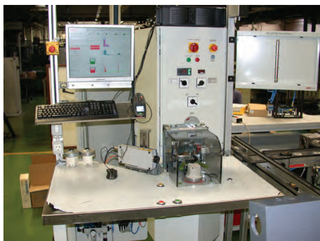
Figure 3: Diagnostic system for total quality control in the new production line of eco-motors at Domel
