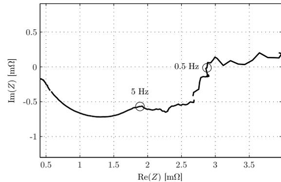
Figure 8: Nyquist plot of the measured PEM fuel cell impedance.
