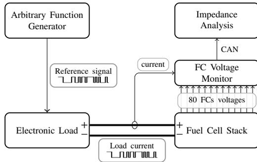
Figure 3: Block diagram of the experimental setup.
