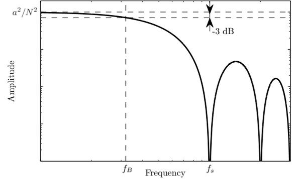
Figure 1: Power spectrum of the PRBS signal.
