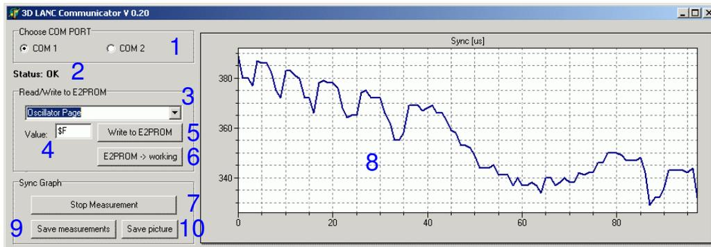
Figure 4. Adjusting parameters of 3D LANC Master and monitoring time disparity can be done by 3D LANC Communicator.
