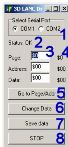
Figure 5. Adjusting of camcorder's and still camera's internal settings can be done by 3D LANC Doctor.
